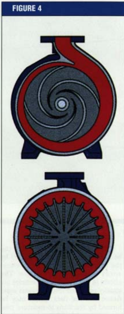
An expanding volute pump (top) and a circular volute pump with a radial vane impeller (bottom).
